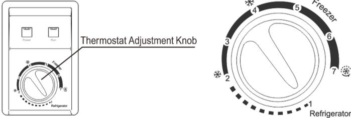
The inside temperature of freezer is regulated by thermostat adjustment knob.
